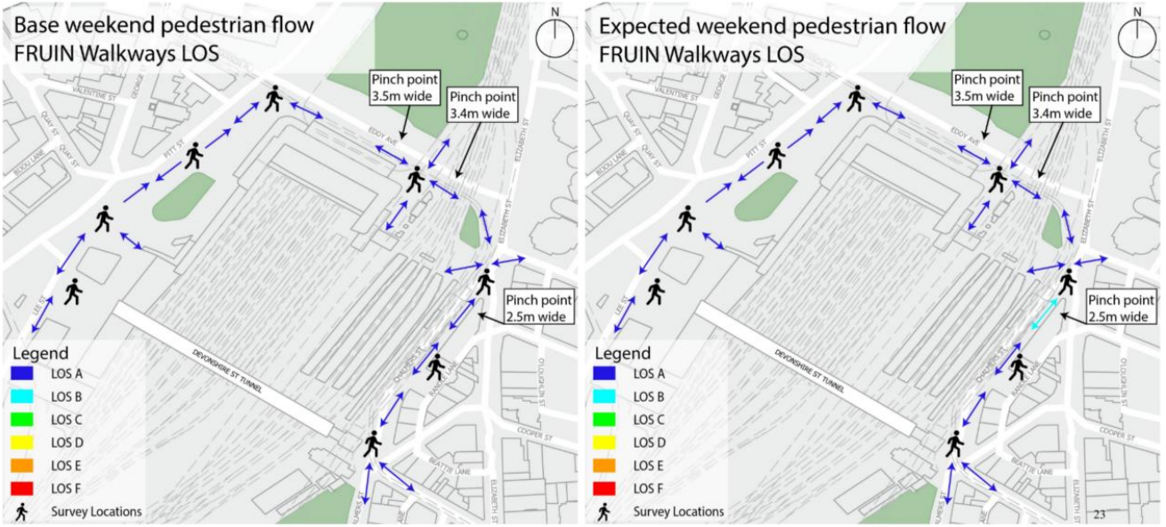
Figure 1-7b: Devonshire St Tunnel pedestrian modelling snapshot
